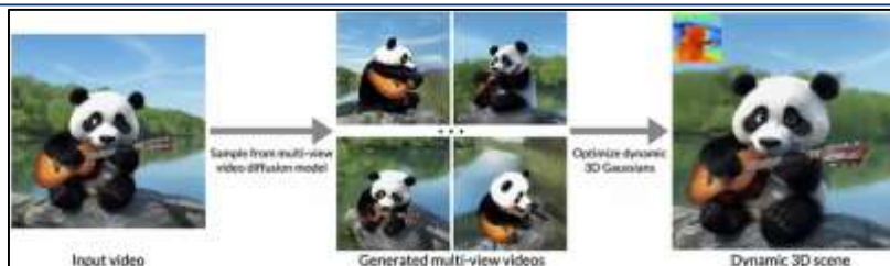
Figure 4: Illustration of the method. Given a monocular video (top), we generate the missing frames (orange frames) of virtual stationary video cameras positioned at all input poses (gray circles) and novel poses (blue circles) using our multi-view video diffusion model. These frames are then used to reconstruct the dynamic 3D scene as deforming 3D Gaussians. Note that although the input trajectory is visualized with changing viewpoints, our method also works for fixed-viewpoint videos.
